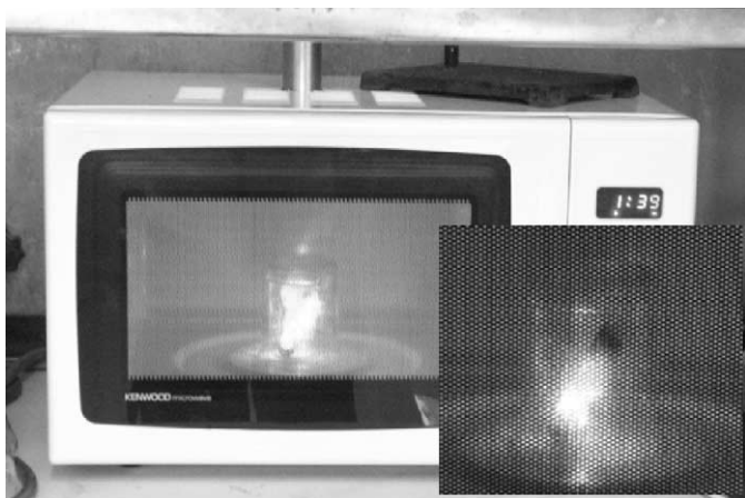
FIG. 1. Photographs of the reaction for the preparation of one of Zintl compounds ( \text{K}_4\text{Sn}_2\text{Se}_6 ) taken during microwave reaction. Insert: higher magnification image.
